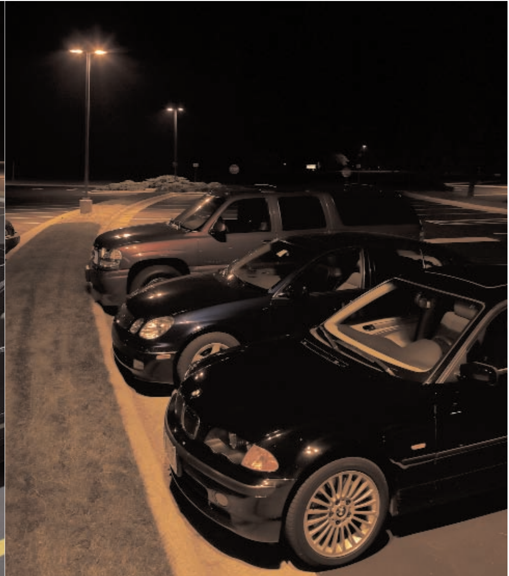
Color rendition under high pressure sodium (21,000 Initial delivered photopic lumens - 300 system watts - 22 CRI)
